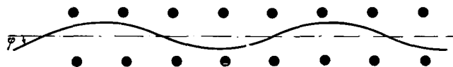
FIG. 1. Schematic representation of a channel and a trajectory of a particle moving in the channel (the image of the trajectory is strongly compressed in the horizontal direction).
