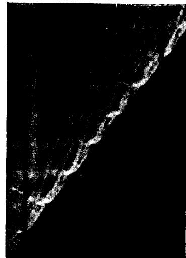
FIG. 13. Photograph of spin detonation in a mixture of 20% H 2 and 80% air on a moving film. The detonation is propagating from left to right and the film is moving from top to bottom.
