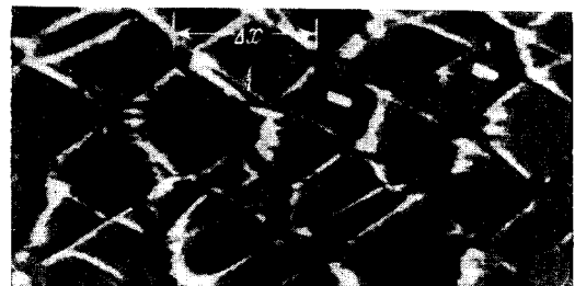
FIG. 20. Imprint left by a pulsating detonation on the lateral surface of the tube.
