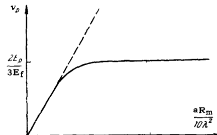
FIG. 11. Number of Frenkel pairs formed at an energy E_p , as a function of the dislocation density 1/\lambda^2 .
