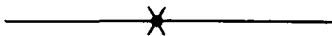
FIG. 4. Feynman diagram describing the correction to the hadron mass due to the medium strong interaction. Solid line — hadron; cross — contribution of the medium interaction, depending on the hypercharge.
