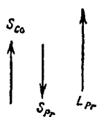
FIG. 48. Dependence of the magnetic moment of \text{Co}_5\text{R} compounds on the magnetic moment of the rare-earth ion.
