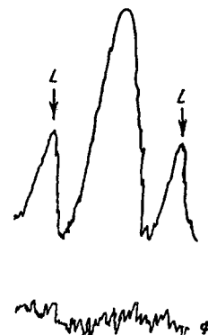
FIG. 6. Microphotogram of the spectrum of the fine structure of the scattered line in glycerine [33] at -27° C. Longitudinal doublet. L - Mandel'shtam-Brillouin components; Φ - background of photographic plate in the neighborhood of the lines.
