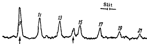
FIG. 2. Combination-scattering rotational spectrum of gaseous oxygen at pressure 3 atm. Grating "ghosts" are marked with arrows.
