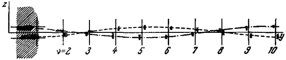
FIG. 20. Results of experimental investigation of axial oscillations of electrons. The dashed areas show the location and size of the luminous spot on the screen as the latter moves along the y axis. The left spot on each orbit is associated with electrons from the outer emission zone, the right spot with those from the inner. The y axis coincides with the common diameter of the orbits, the z axis is perpendicular to the plane of the orbits. The vertical lines show the theoretical positions of the points of intersection of the corresponding orbits with the y axis.
