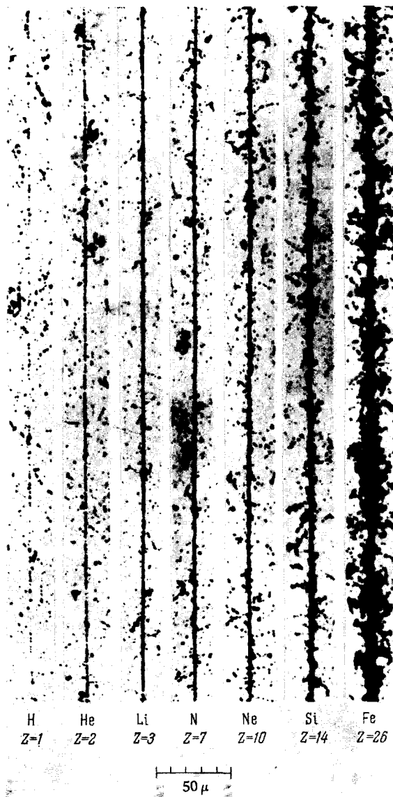
FIG. 1. Emulsion tracks of relativistic nuclei with different Z . It is seen that the thickness of the track increases with increasing Z .
