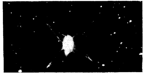
FIG. 14. Nucleation of domain walls around an artificially introduced defect. [15]
