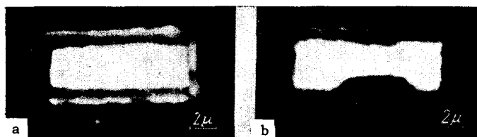
FIG. 18. Cross section of an oxidized iron whisker. [15]
