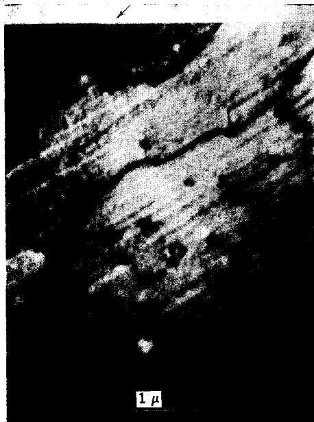
FIG. 3. Electron micrograph showing narrow deformed zone immediately after its formation in a zinc whisker. The zone boundaries are indicated by arrows. Pyramidal slip traces and dislocations are visible within the zone. [30]
