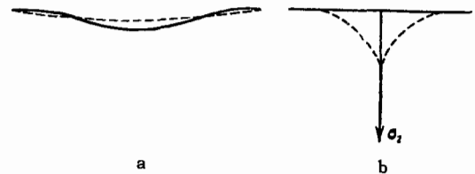
FIG. 13. Schematic nature of the "smoothing out" of a scratch on the surface of a crystalline body (a), and of the development of a thermal etching groove at the place where an intergrain boundary meets the surface (b).
