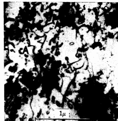
FIG. 36. Aluminum deformed by fatigue ( 1.4 \times 10^6 cycles). [58]
