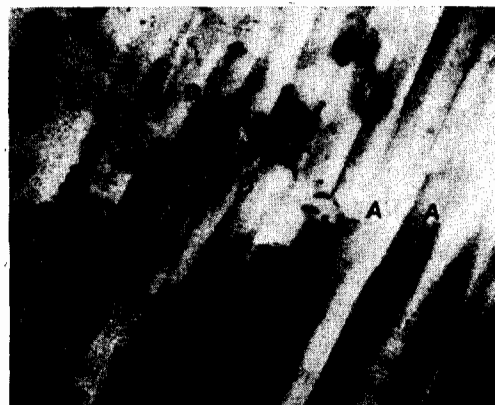
FIG. 14. Movement of dislocations in aluminum foil. Curved paths (cross slip) are visible. [65]
