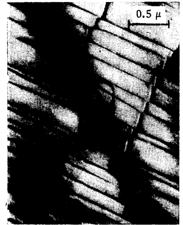
FIG. 12. Double image of one of two types of interacting dislocations in Al. [28]
