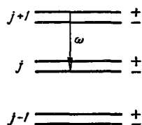
FIG. 2. Splitting of rotational levels into two inversion sublevels. The arrow indicates an allowed transition.
