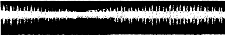
FIG. 11. Example of record of the rotational Doppler effect in Moscow, in the case when additional amplitude modulation due to the effect of small-scale irregularity in the ionosphere is observed.
