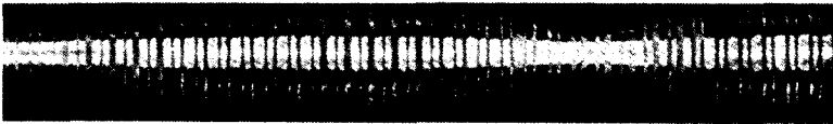
FIG. 9. Example of record of amplitude modulation of the radio signals of the third satellite, due to the Faraday rotation; Moscow, 1958.
