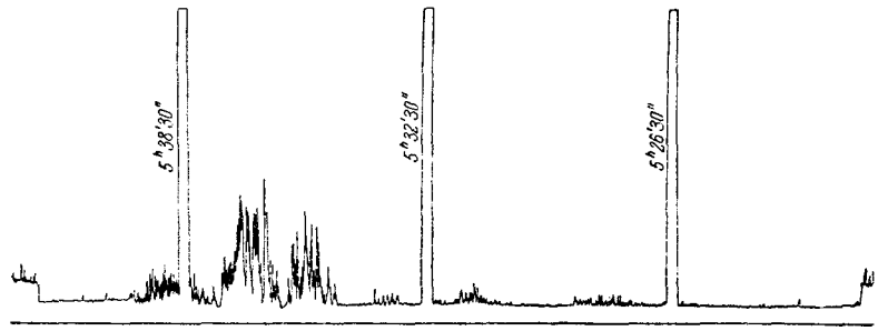
FIG. 17. Example of record of the amplitude of radio signals from the third satellite, made in Moscow, where multiple-reflection reception of radio signals from 8,000 or 10,000 km away was observed.
