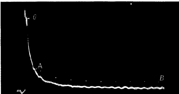
FIG. 4. Oscillogram showing the time decay of the flux of neutral atoms.
