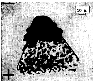
FIG. 1. A coarse emulsion microcrystal showing a print-out effect displaced in an electric field.
