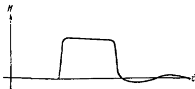
FIG. 26. Shape of the pulsed magnetic field.
