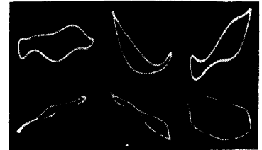
FIG. 10. Various phase positions of a distorted sinusoidal-sweep figure, frequency ratio 1:1.
