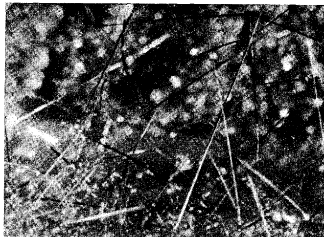
FIG. 3. Copper whiskers (Brenner) from the reduction of CuI ( \times 20 ).
