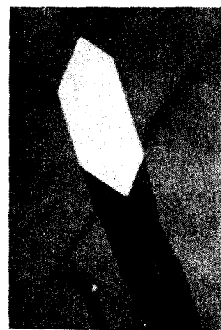
FIG. 5. Hexagonal cross section of whisker ( \times 60 ).
