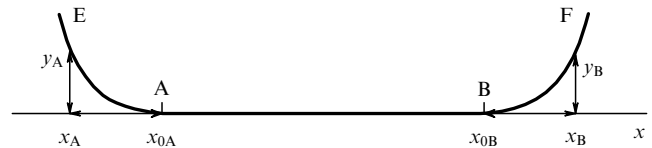
Figure 4. A diagram illustrating the quantification of curved regions in the grain boundary (GB) near the (100)_{\Sigma 3 \text{ CSL}} facet. This diagram has been reproduced from [73] with the permission of the American Physical Society © 2004.
