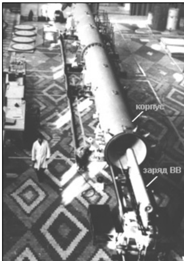
Explosive photodissociation iodine laser (EPIL) with an active region diameter of 1200 mm and output energy of 1 MJ (for more details, see [1]).
