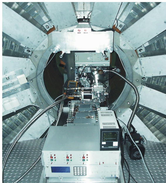
Figure 10. A dual-band (3 and 2 mm) SIS receiver, developed at the IAP RAS in collaboration with the IRE RAS and a number of other organizations, is installed on the 14-meter radio telescope of the Metsahovi Observatory in Finland (2004).
