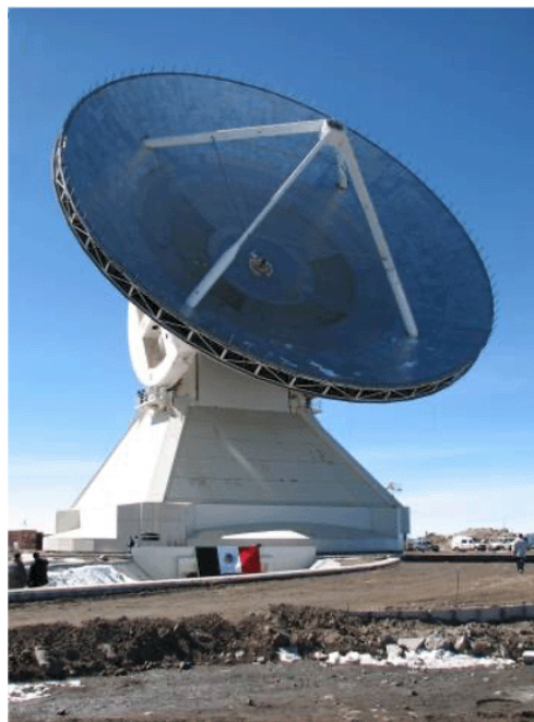
Figure 3. The Large Millimeter Telescope Alfonso Serrano, 50 m in diameter, is located on the summit of the Sierra Negra (4,600 m above sea level) in Mexico. ©LMT.
