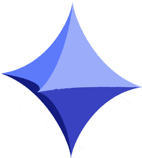
Figure 24. Distorted octahedron modeling the spatial distribution of the velocity of longitudinal acoustic vibrations from the crystallographic direction for cubic crystals [96].
