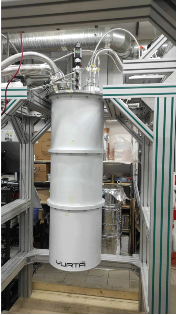
Figure 1. High cooling capacity ^3\text{He} – ^4\text{He} dilution refrigerator.
