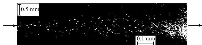
Figure 11. Scattering centers ('sparkles') that appear in \text{LiNbO}_3 crystal in passage of laser radiation through it. Arrows mark entry to crystal and exit of laser beam from the crystal. Photograph is published for the first time.
