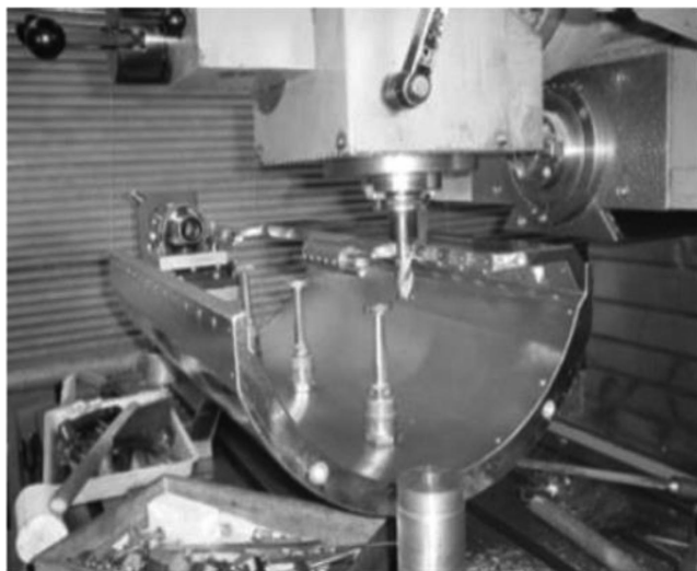
Figure 19. Mounting of accelerating electrodes using a machine.
