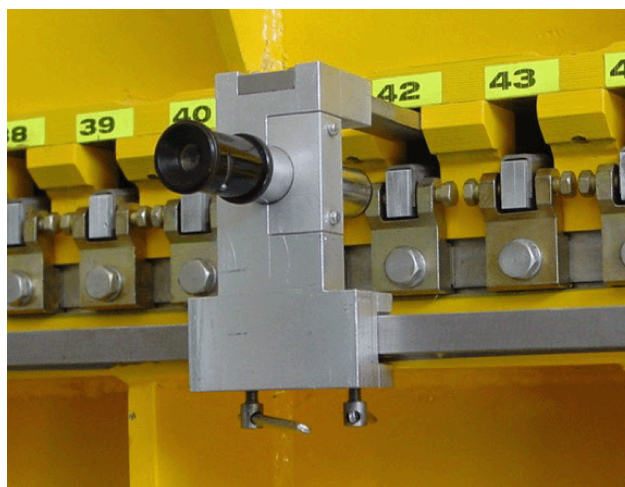
Figure 9. System for adjusting position of magnetic coils to achieve magnetic field rectilinearity at a level of better than 10^{-5} .
