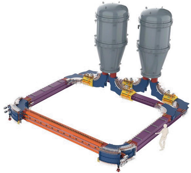
Figure 19. Collider's ECS has two cooling sections with electron beams moving in straight sections towards each other to cool ion beams in NICA collider in upper and lower rings.
