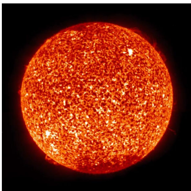
Figure 3. Image of the quiet Sun taken in the 304 Å resonance line of He II ion (a telescope with a multilayer Mg/Si mirror synthesized at the Institute for Physics of Microstructures, RAS) from an Earth satellite on March 1, 2009. Angular resolution is 1.7'' [23].
