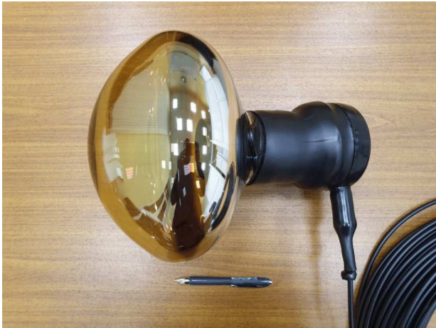
Figure 5. Image of a 10-inch R7801-100 photomultiplier tube [30].
