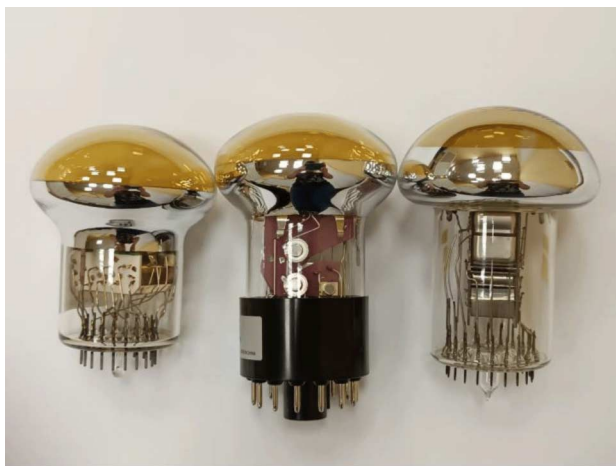
Figure 10. Image of three-inch photomultiplier tubes. From left to right: XP72B20, R14374, and SFERA.
