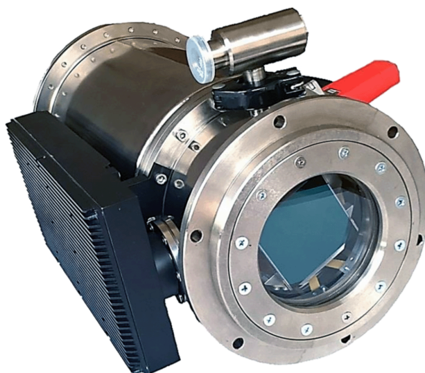
Fig. 11. Cryostated camera with a CCD231-84 photodetector and camera electronics unit.
