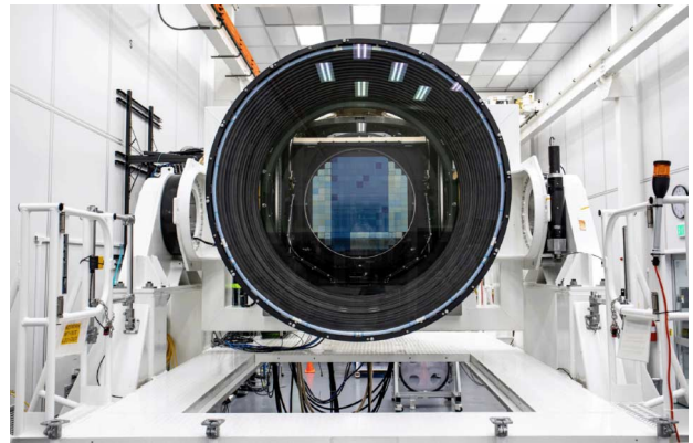
Fig. 7. Mosaic camera for LSST consisting of 3.2 billion elements in an assembly shop.
