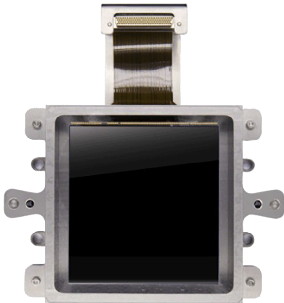
Fig. 8. GSENSE1081BSI CMOS device made of 9K \times 9K elements in a silicon carbide frame.
