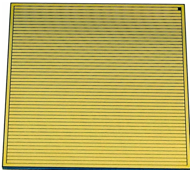
Figure 9. CdTe crystal for the SD01 detector (top view, size: 29.95 × 29.95 × 1.00 mm).
