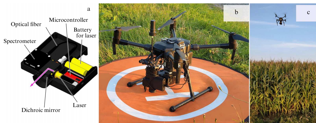
Figure 2. (a) Schematic of a compact fluorescent lidar instrument. (b) Photograph of a fluorescent lidar device mounted on a drone. (c) Photograph of the process of measuring a corn field from a drone equipped with a fluorescent lidar device.
