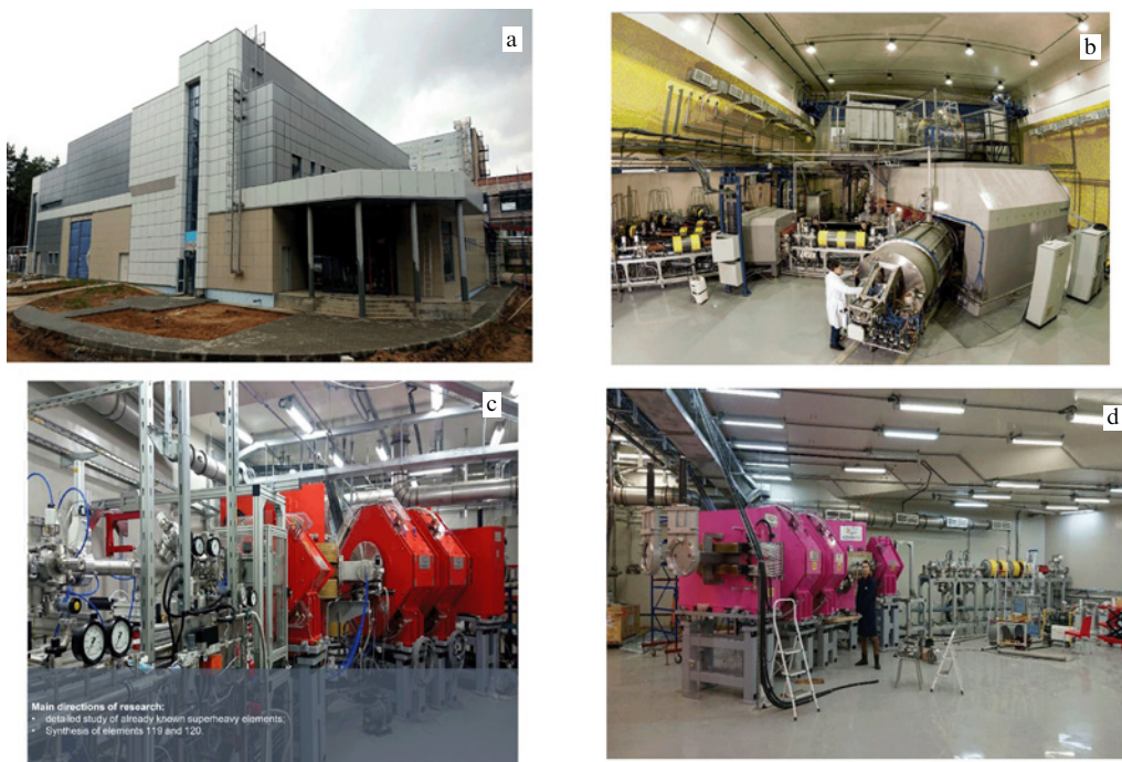
Figure 8. (a) Superheavy Element Factory of JINR FLNR in Dubna was commissioned in 2018. (b) New DC-280 cyclotron of JINR FLNR. (c) Gas-filled recoil separator — DGFRS-2. Research areas: detailed study of already known elements and synthesis of new superheavy elements 119 and 120. (d) Gas-filled recoil separator — GRAND (DGFRS-3). Research areas: nuclear and mass spectroscopy of superheavy elements and study of their chemical properties.
