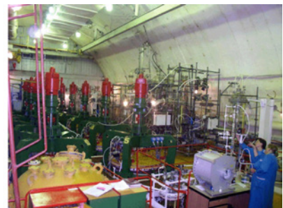
Gallium-germanium neutrino telescope (Baksan neutrino observatory of INR RAS) is a facility containing a 50-ton metal-gallium target, which is installed in a low-background laboratory in an underground mine with a volume of 7,000 m³ at a depth of 4,700 meters of water equivalent (3,500 meters from mine portal).
