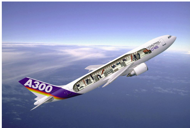
Figure 3. Airbus for parabolic flights within the joint programs of the European Space Agency and the German Aerospace Center. On board, there is a scientific laboratory and the TEMPUS facility aimed to measure thermophysical and kinetic properties of liquid metals, as well as crystallization kinetics of metallic, semiconductor, and alloy samples.
