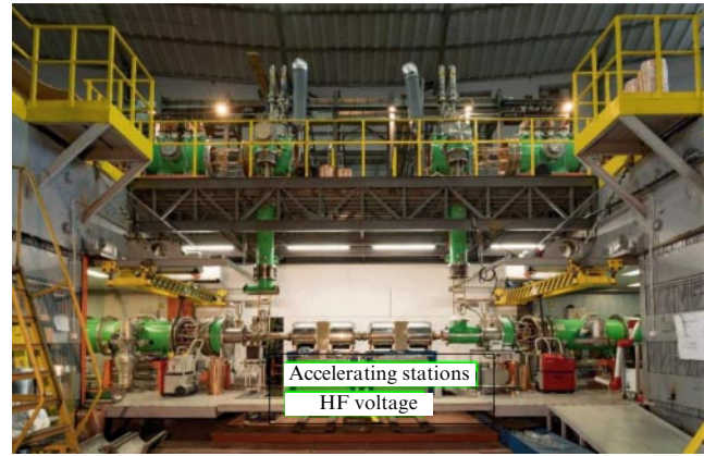
Figure 3. Accelerating stations of the booster in the second straight gap. Elements of the measuring section are installed on the overpass, including a dipole magnet, a doublet of quadrupole lenses with inductive field sensors, high-current current leads, and an input of cryogenic liquids.
