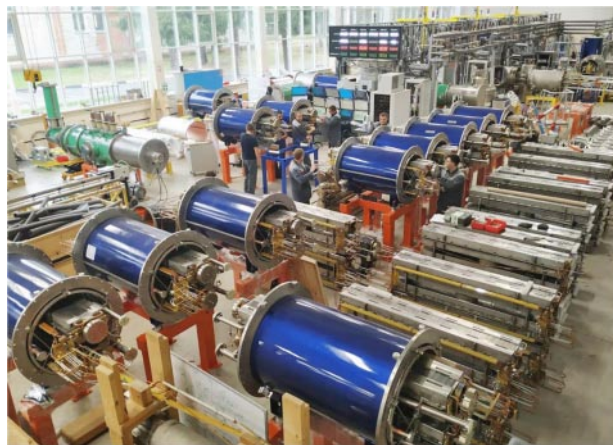
Figure 8. Superconducting magnet assembly and testing line.
