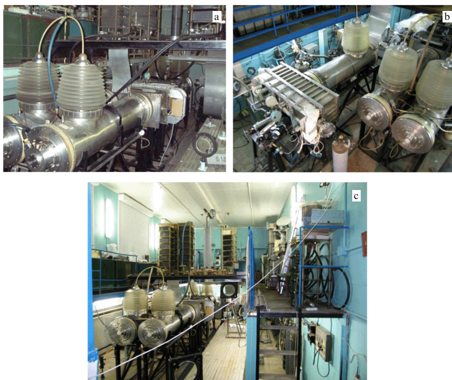
Figure 12. Photos of the GARPUN KrF laser: main amplifier (a), preamplifier (b), and general view of the facility (c).
