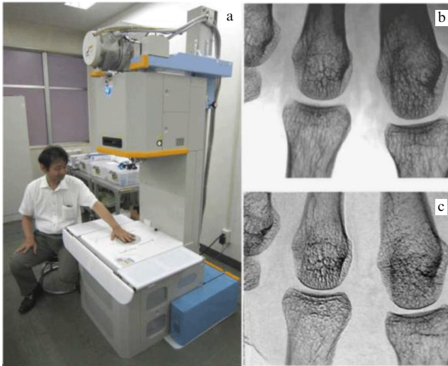
Figure 17. Talbot–Lau system for X-ray phase visualization installed in a hospital (a) and the obtained absorption image (b) and dark-field image (c) of a part of a palm of the first author of Refs [309, 310].
