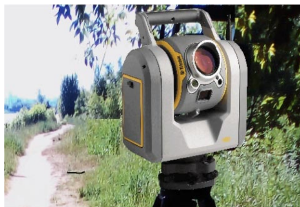
Figure 13. (Color online.) Robotized Trimble SX10 electronic tachometer installed on a track passing parallel to the Skhodnya Canal (left of the track) [98].
