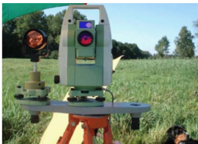
Figure 5. Robotized Leica TCRP1201 electronic tachometer with a corner reflector mounted on a horizontal plate at instrument height [69].
