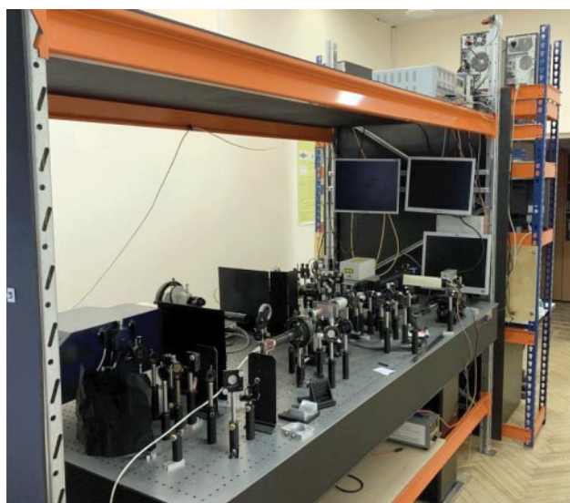
Figure 5. Photograph of the setup for laser heating of substances in high-pressure cells.
