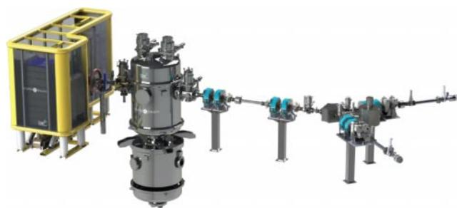
**Figure 21.** (Color online.) Neutron generator with a low-energy beam path, the tandem accelerator, a high-energy beam path, and a system for distributing the beam through channels at the neutron-generating target in rooms for patient irradiation.
