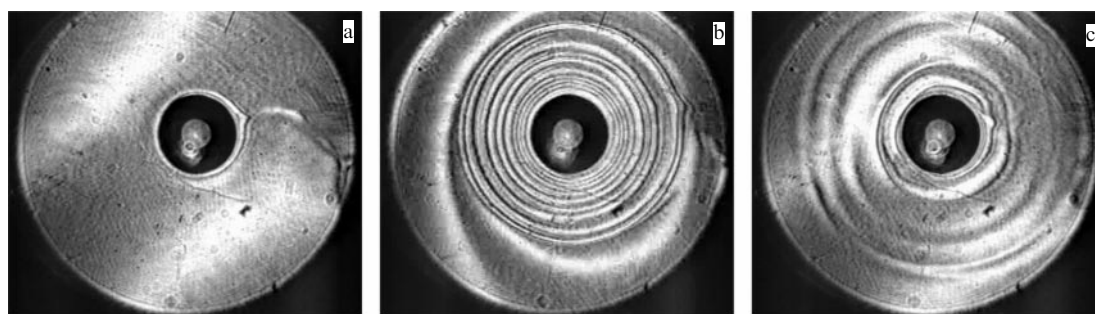
Figure 2. Evolution of the concentration field perturbation around an air bubble in a horizontal layer of an aqueous solution of isopropyl alcohol. Layer thickness h = 2.6 mm, concentration difference \Delta C = 20\% , bubble diameter d = 5.0 mm. Top view: (a) t = 0 , (b) t = 2.0 s, (c) t = 10.0 s.
