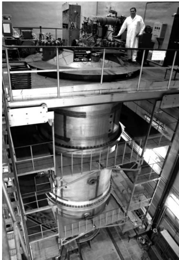
Figure 8. Electrostatic charge exchange generator (tandem) EGP-10, operating energy range of accelerated protons from 1.0 to 12 MeV; types of accelerated particles: ions of protium, deuterium, tritium, oxygen, carbon; source of negative ions is a duoplasmatron. (Photo by A E Maleev.)
