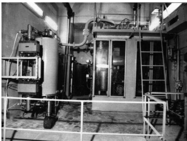
Figure 18. LU-10-20 linear resonance accelerator designed to simulate the dose effect of gamma-ray radiation. (Photo by V A Razuvaev.)
