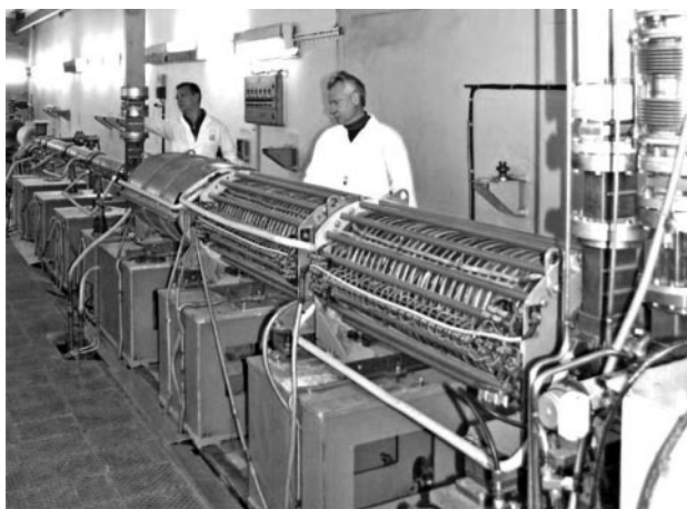
Figure 7. LU-50 electron accelerator. Boundary electron energy is 50 MeV, photoneutron energy ranges from 0.1 to 15 MeV (made jointly with the Moscow Radio Engineering Institute). (Photo by V A Razuvaev.)
