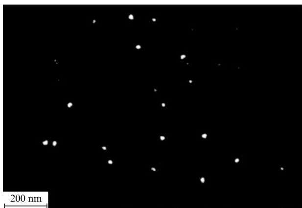
Figure 13. Transmission electron microscopy image of the \text{Al}_{88}\text{Ni}_6\text{Y}_6 alloy after cryogenic thermocycling [122].
