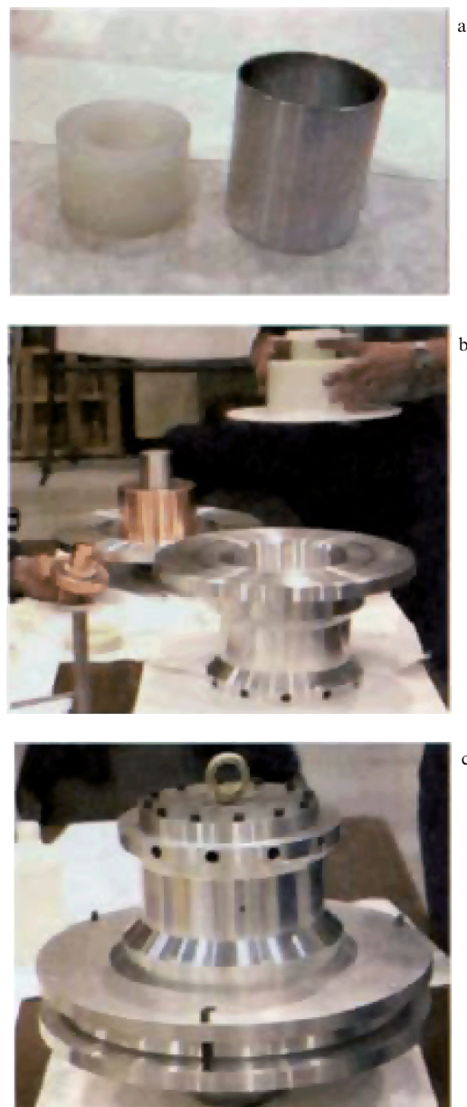
Figure 29. (Color online.) Cylindrical liner PU for RUS-6, 7 experiments at the ATLAS facility for studying the dynamic strength of copper. (a) Outer (current-carrying) Al liner of radius R = 31 mm and thickness \Delta = 2 mm. On the left is an intermediate polyethylene layer of a three-layer liner system. (b) PU assembly process. On the right (in the hands) is a part of a PU with a Cu liner, on which axisymmetric initial perturbations are applied. (c) PU assembly with a reverse current line.
