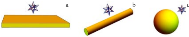
Figure 6. Geometries of the problem of spontaneous emission of an EQS, where there is an exact analytical description: (a) lamellar (layered) structures, (b) circular cylinder, and (c) spherical nanoenvironment. Star denotes EQS.
