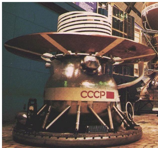
Figure 4. (Color online.) The Venera 13 spacecraft during laboratory tests. The TV camera entrance closed with a lid is located at the top of a spherical body over the inscription СССР. A spiral omnidirectional transmission antenna is located over a round shield decelerating the spacecraft's descent in the dense atmosphere of the planet. The landing buffer below absorbed the shock energy during landing. The ring to the right over the landing buffer is the antenna of the Groza instrument which detected electric discharges in Venus's atmosphere. The spacecraft height up to the circular parachute shield is 1 m.
