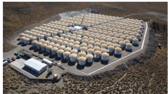
Figure 4. HAWC facility near Pueblo, Mexico located at an altitude of 4,100 m above sea level (Sierra Negro volcano). Individual detectors are water-filled tanks for registering Cherenkov radiation of EAS particles. It is essentially an implementation of Cocconi's idea dated 1959 [4].
