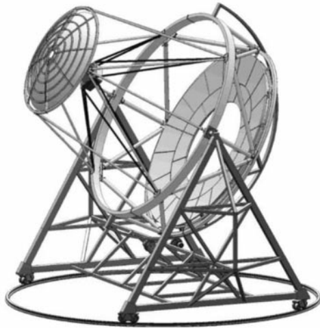
Figure 5. View of an optical system with two mirrors (the Schwarzschild–Couder telescope) designed for the AGIS project.
