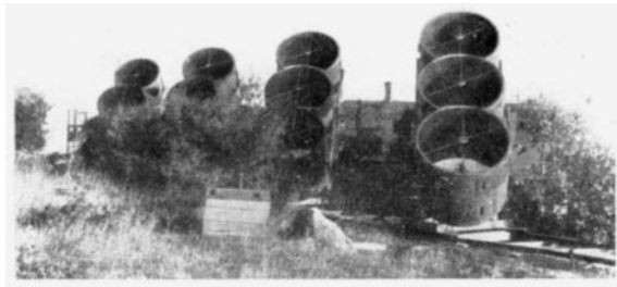
Figure 1. First Cherenkov gamma-ray telescope (and gamma-ray telescope in general), built by A E Chudakov and collaborators in the Crimea.
