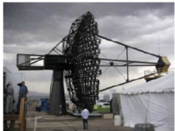
Figure 3. A VERITAS array reflector: a typical third-generation Cherenkov telescope.
