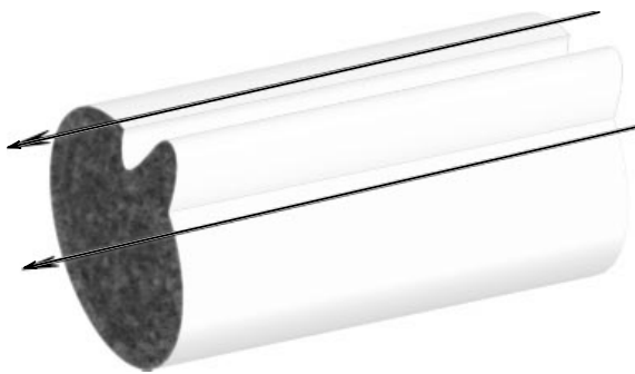
Figure 2. Perturbation of plasma boundary associated with the development of flute instability. Arrows show main magnetic field lines.
