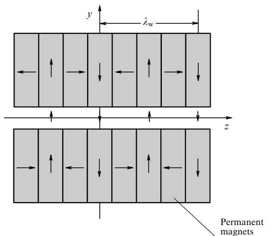
Figure 15. Plane undulator with permanent magnets.
