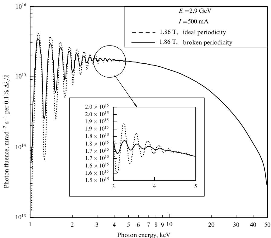
**Figure 19.** Spectrum of radiation from a multipole wiggler with a small field period.
