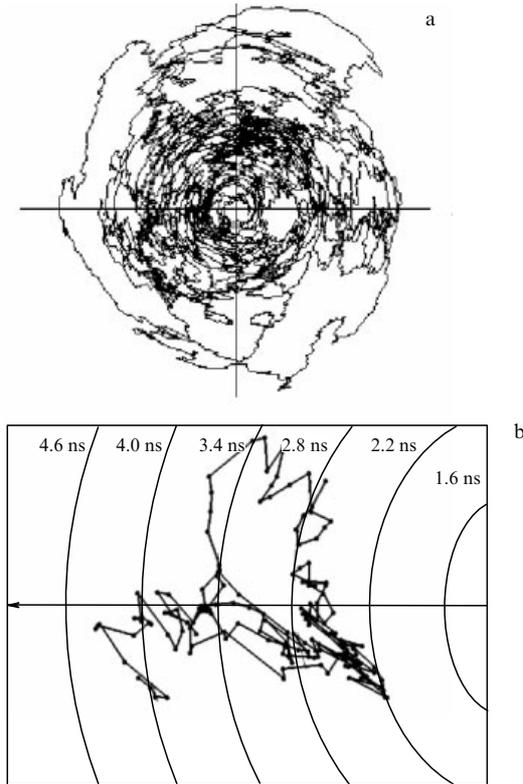
**Figure 17.** (a) Electron trajectory on the phase plane of longitudinal motion. (b) Close-up of the phase trajectory part from Fig. a.
