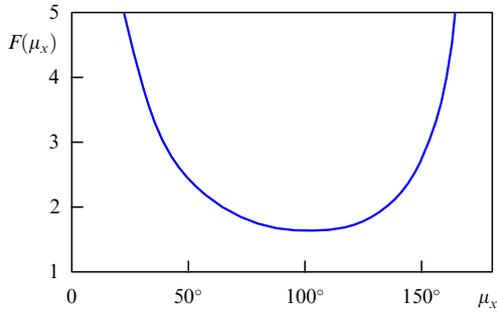
**Figure 24.** Function  $F(\mu_x)$  in (63) versus the betatron phase shift over the FODO cell.
