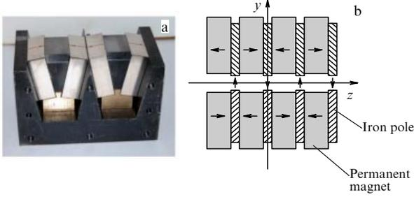
**Figure 12.** (a) Model of an undulator with permanent magnets (lower part of an undulator) without sidewalls. Wedge-shaped iron poles allow concentrating the magnetic flux and increasing the amplitude of the field in the gap. (b) Scheme of a hybrid undulator.
