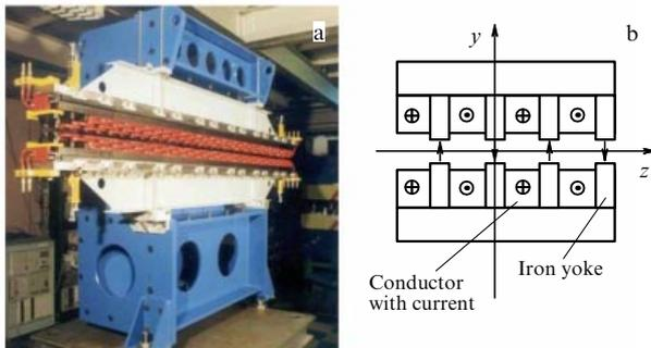
**Figure 13.** (Color online.) (a) Electromagnetic undulator (coils are in red). (b) Diagram of the electromagnetic undulator cross-section.
