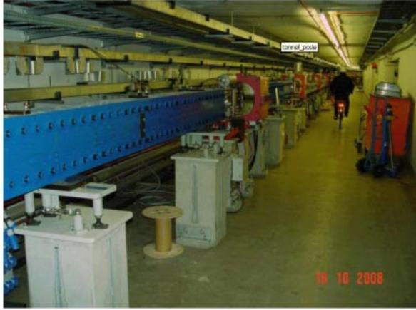
Figure 20. Damping wigglers installed at the PETRA III SR source.
