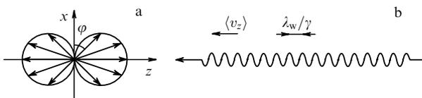
**Figure 11.** Undulator radiation in the comoving reference frame. (a) Directivity pattern of dipole radiation (more precisely, its cross section by the  $xz$  plane). The length of the arrows whose ends are located at the circles are proportional to the amplitude of the radiation field in the corresponding direction. (b) Undulator field approaching an electron with the speed  $\langle v_z\rangle$ .
