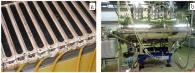
**Figure 18.** Superconducting wigglers fabricated at the INP SB RAS. (a) part of a yoke from a multipole wiggler with a small period used at Canadian Light Source (CLS). (b) Wiggler with a large field amplitude in a cryostat for SR source Sibir 2 (NRC “Kurchatov Institute”).
