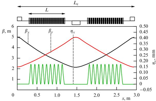
**Figure 23.** Two wigglers with a length  $L$  installed in the FODO optical cell with a length  $L_c$ . The plot shows betatron functions and the dispersion function  $\eta_x$  calculated using MAD8 software (<http://mad8.web.cern.ch/mad8/>).
