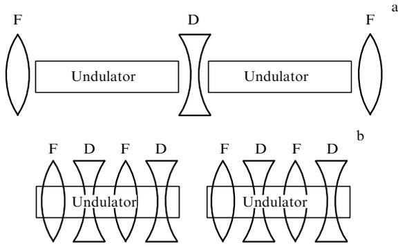
**Figure 21.** FODO-cell for placing wigglers and undulators with separated (a) and combined (b) functions.
