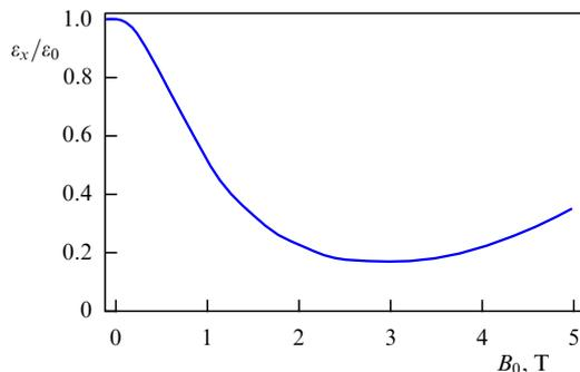
**Figure 22.** Relative variation of the beam emittance caused by the wiggler influence.
