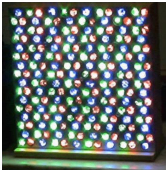
Figure 18. Exterior view of a full-color video module: 8 \times 8 pixels (192 lamps).
